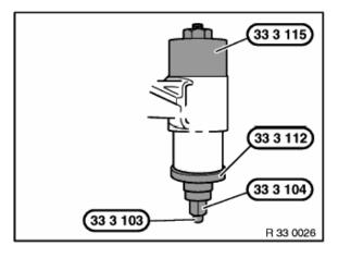
Coat new rubber mount with Circolight (refer to BMW Parts Service) and pull in with special tool 33 3 103/104/112/115.
