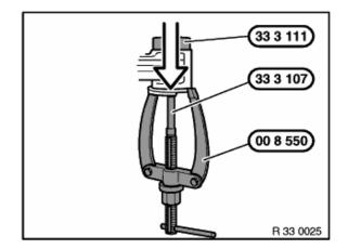
Pull out rubber mount using special tool 00 8 550/33 3 107/111.
